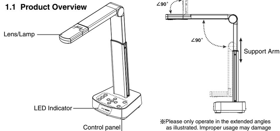
※Please only operate in the extended angles as illustrated. Improper usage may damage the machine.
